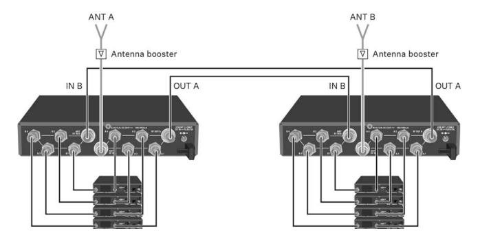
Option 3: Two antennas supply a 8-channel system
