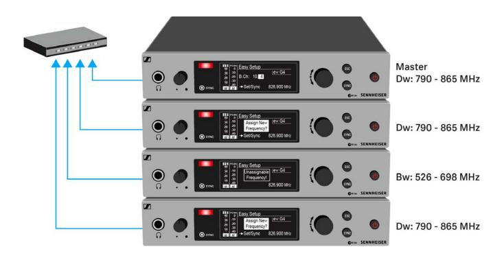
Select an unused frequency for one of the connected receiver on the master receiver.
