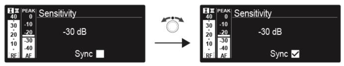
When the check box is activated, the value will be transmitted during synchronization. If it is deactivated, the value will not be transmitted.
