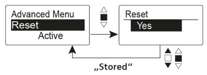
When you reset the wireless microphone, only the selected settings of the pilot tone and the **U1** to **U6** frequency banks are retained.
