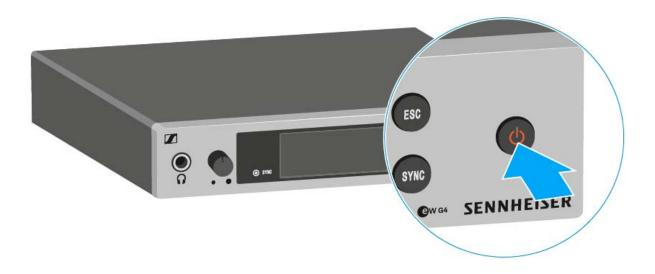
To switch the receiver to standby mode:
