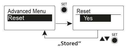
When you reset the bodypack transmitter, only the selected settings of the pilot tone and the **U1** to **U6** frequency banks are retained.
