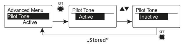
The pilot tone has an inaudible frequency that is sent from the transmitter and evaluated by the receiver. It supports the receiver's squelch function.
