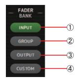
Allows you to select which fader bank is displayed in the channel strip area ( $\rightarrow$ page 11).
